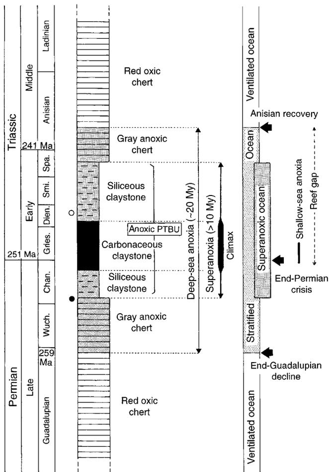
**Fig. 3.** Stratigraphic column of the P-T boundary section in deep-sea chert facies of Panthalassa. Note the symmetrical change in lithostratigraphy and redox condition across the boundary, and quick biotic responses to environmental changes. The solid and open circles represent stratigraphic horizons of the youngest Permian and the oldest Triassic microfossils, respectively.
